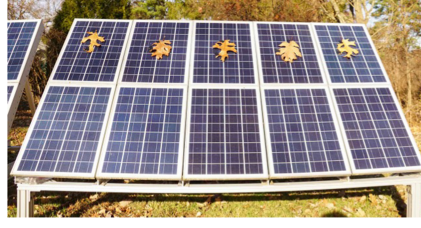
Fig. 7. A synthetic leaf occlusion fault in our experimental array.
