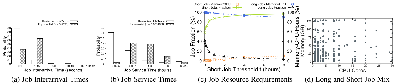
Fig. 15. Histograms of job inter-arrival times (a) and service times (b) for our real production batch workload along with an exponential distribution using the same mean, as well as the mix of long and short jobs (c) and a scatterplot of job resource requirements (d).
